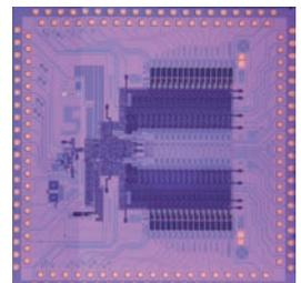
A 1 cm<sup>2</sup> chip, fabricated with HYPRES' standard Nb process with  $J_c = 4.5$  kA/cm<sup>2</sup>, contains a bandpass delta-sigma ADC, a digital channelizer, and output drivers.
