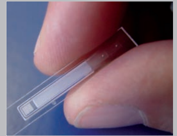
example of a microcooler developed at the University of Twente, Netherlands.
