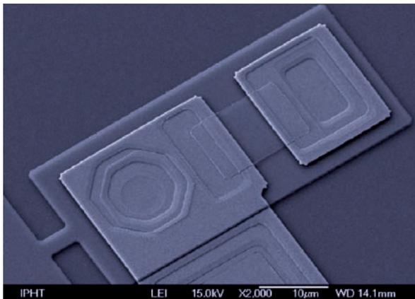
The basic active device of superconducting electronics: a Josephson junction. This picture shows a resistively-shunted Josephson junction made from a Nb/AlO<sub>x</sub>/Nb trilayer, working at 4.2 K for high speed digital applications - Source: Fluxonics Foundry
