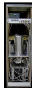
A complete cryocooled digital-RF receiver system prototype, assembled in a standard 1.8-meter tall 0.5-meter wide equipment rack. Using the modular packaging approach, the system can currently host variety of chips, such as the one shown in the previous picture. The system includes a two-stage 4-K Gifford-McMahon cryocooler manufactured by Sumitomo, two sets of interface amplifiers for connecting chip outputs to an FPGA board (placed behind the vacuum enclosure, on the metal tray) for further digital processing and computer interface. The system also includes a current source and a temperature controller.
