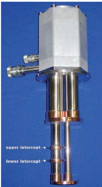
*Two stage pulse tube cooler with heat interceptors
