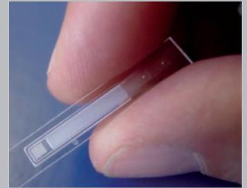
example of a microcooler developed
