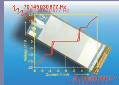
The 10V series array developed at PTB consists of 69,632 overdamped Josephson junctions, where the number of junctions follows a binary sequence. The area of each junction amounts to  $12 \mu\text{m} \times 30 \mu\text{m}$ . The size of the whole chip is approximately  $10 \text{ mm} \times 24 \text{ mm}$ . A constant-voltage step at the 10-V level is generated under microwave irradiation at 70 GHz.
