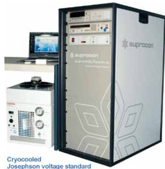
Figure 1: Photograph of "supraVOLTcontrol"
